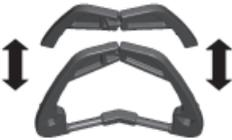
To pry open the connecting joint at the opening, carefully and repeatedly move the hanger brackets in opposite directions.
